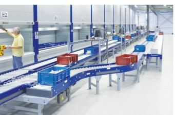
For quick order picking and consolidation of orders, work zones can be easily connected via conveyor systems. Items are delivered automatically to the access opening, picked and then placed into shipping containers on the conveyor. As orders are completed, the containers can be directly routed to shipping via conveyor for a fast and trouble-free operation.
