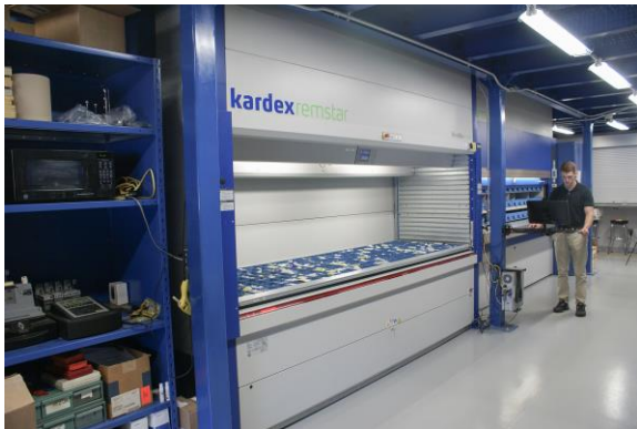
Vertical Carousel & Shuttle VLM technology at work in a parts department
