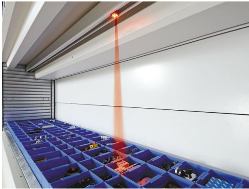
Pick to Light Technology: Light Pointer
