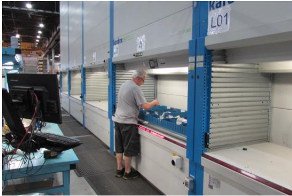
Shuttle VLMs support order fulfillment in a distribution facility
