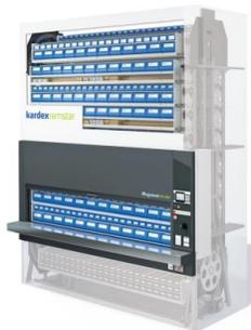
**Vertical Carousels** – Comprised of a series of shelves that rotate around a track—similar to a Ferris wheel—these automated storage and retrieval systems quickly deliver stored items to an ergonomically positioned work counter at the operator's command. When compared to static shelving and rack, they save up to 75% of floor space.
