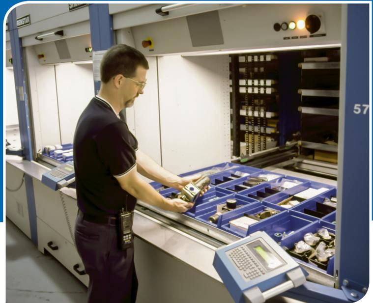
BMW figures their Shuttle VLM system holds the equivalent of 45 drawer cabinets in half the floor space.
