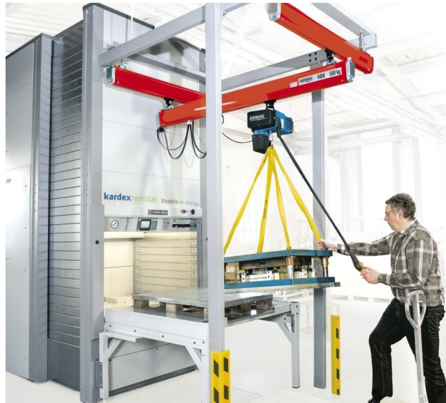
Shuttle XP VLM with Crane Handling in Action
