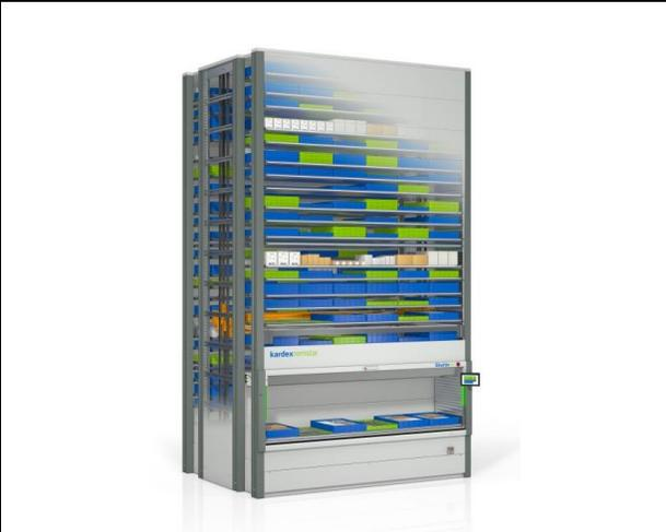
**Vertical Lift Modules (VLMs)** – An enclosed system with two columns of trays and a central inserter/extractor that automatically finds and pulls trays from both columns, then presents them to the operator.
