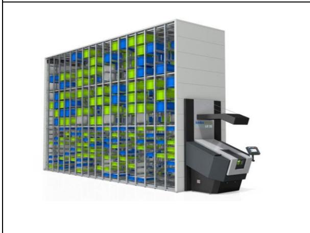
**Vertical Buffer Modules (VBMs)** –In the middle of a multi-segment shelving system is an aisle, where a moveable mast with a telescopic gripper operates. The control unit sets the gripper in motion picking a bin and transporting it to a picking station.
